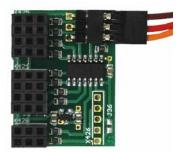
Nautic/Multiswitch at X3 must be activated in the Drive-Teacher under **Configuration** → **Nautic/Multiswitch**.
