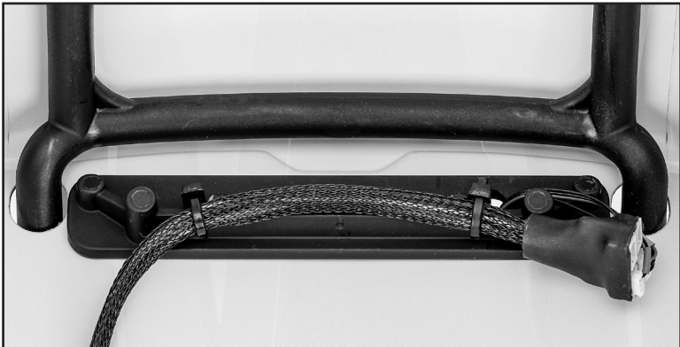
Rear Light Bar Wiring/Long Extension Harness installed on Rear Light Bar Mount
