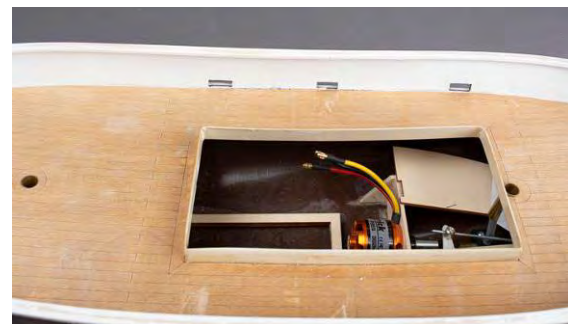
Fig. scuppers made and deck placed
