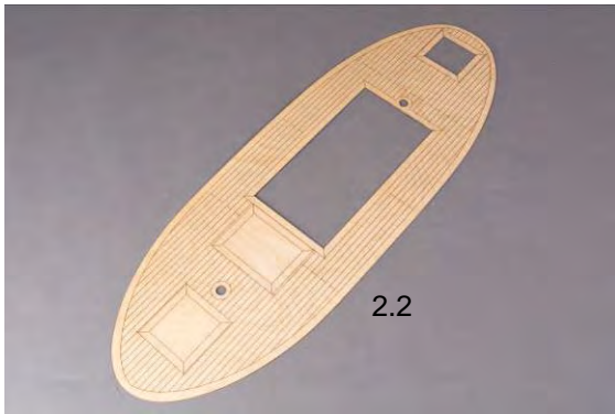
Fig. laser engraved plywood deck
