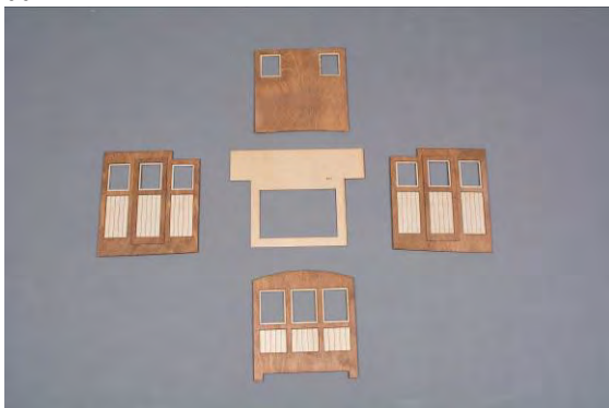
Fig. superstructure parts stained and glued
