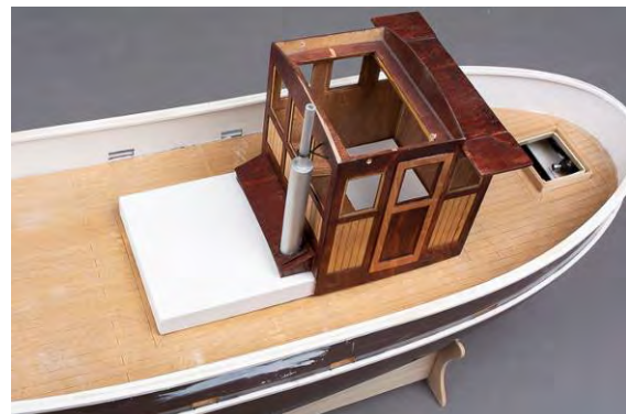
Fig. Position the superstructure on the hull
