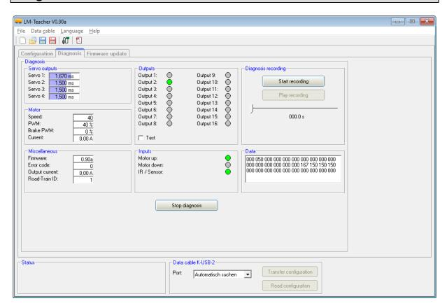
A diagnostic function is integrated in the LM-Teacher. This feature is very helpful to check the various functions of the light module. The data cable K-USB-2 must be connected to X5/7 at the light module.
