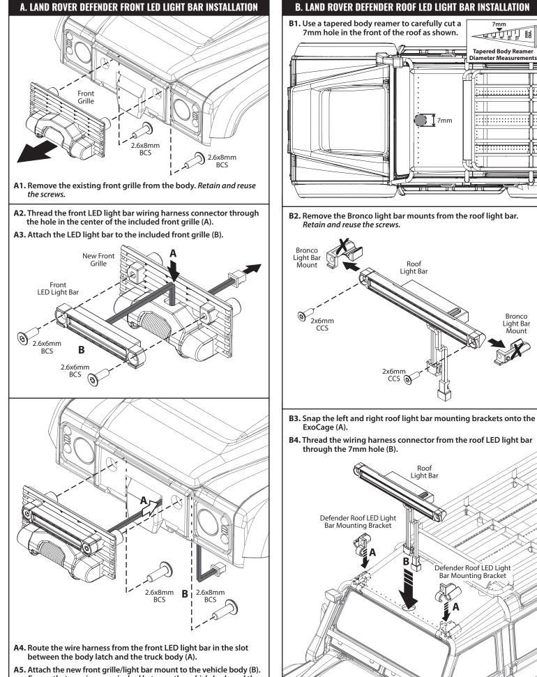
Ensure that no wires are pinched between the vehicle body and the front grille before tightening the screws.
