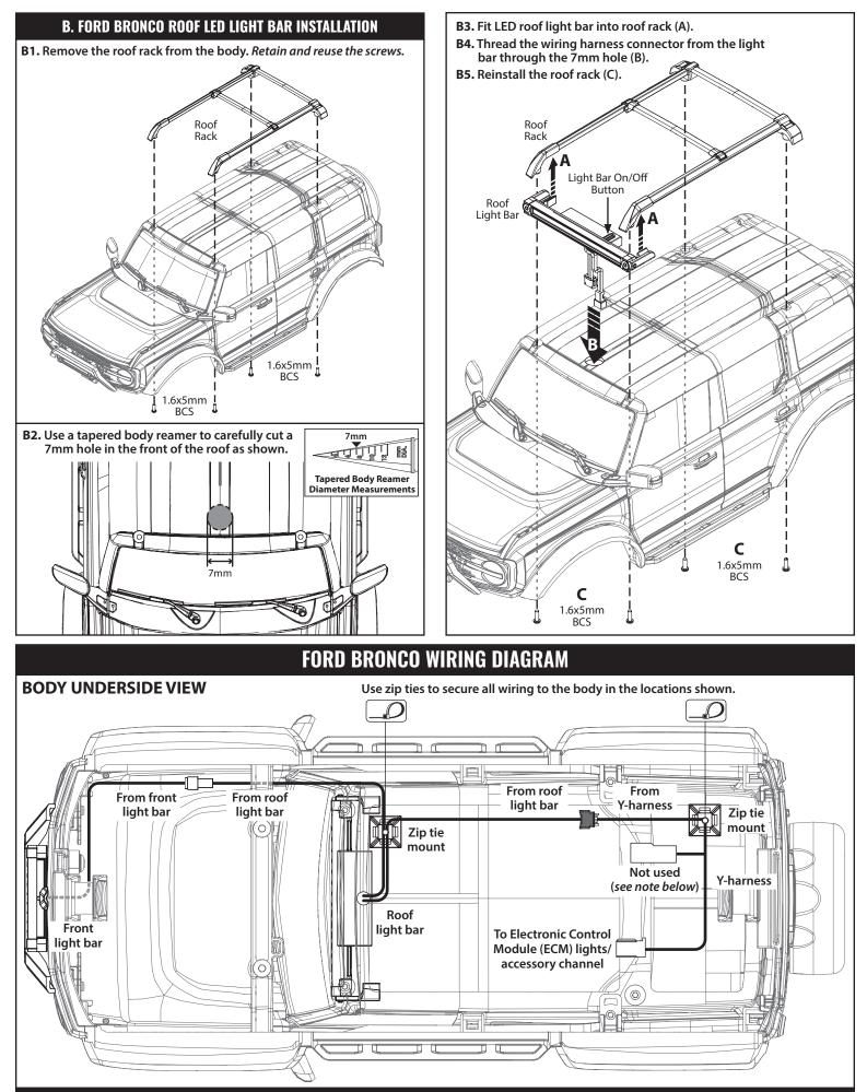
Note: If the #9783 body light kit has been installed on the body, plug the #9783 connector into the included Y-harness.
