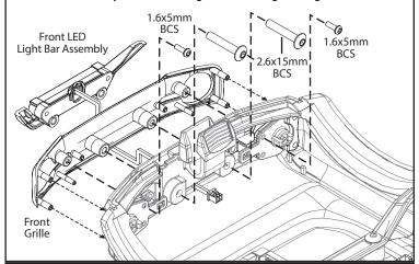
Note: The 2.6x15mm BCS will break through the grille during installation.
