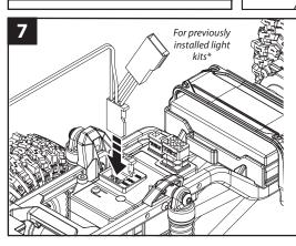
Plug the Y-harness into an open ACC port on the electronic control module (ECM). The LED lights will turn on when the ECM is powered on by plugging in the battery.
