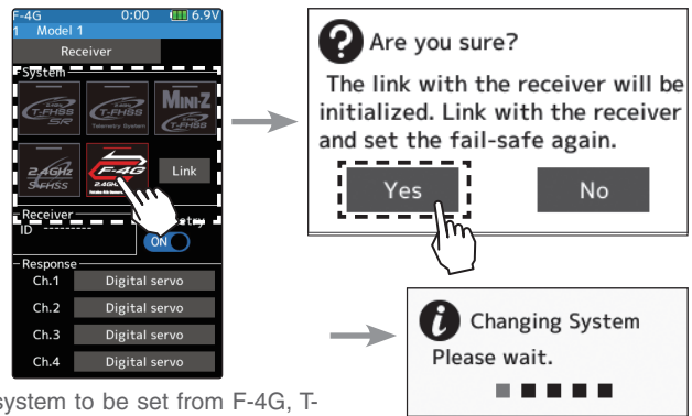
Tap the system to be set from F-4G, T-FHSS SR, T-FHSS, S-FHSS or Mini-Z.
