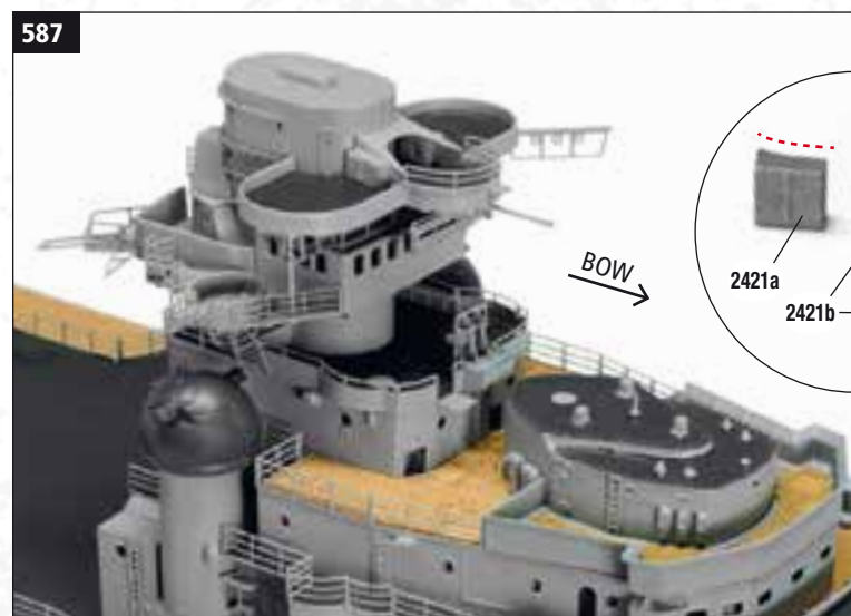
587 Once dry, take the tower structure and glue it on the upper navigation deck, as shown in the picture.
