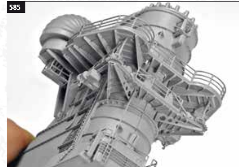
585 The picture shows the assembly of cable 1008 with bracket 1009 seen from another angle.
