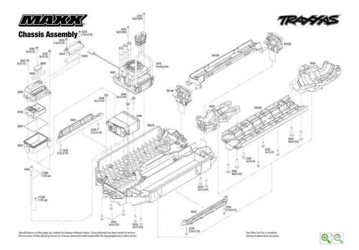
Maxx® (89086-4) Chassis Assembly Exploded View
